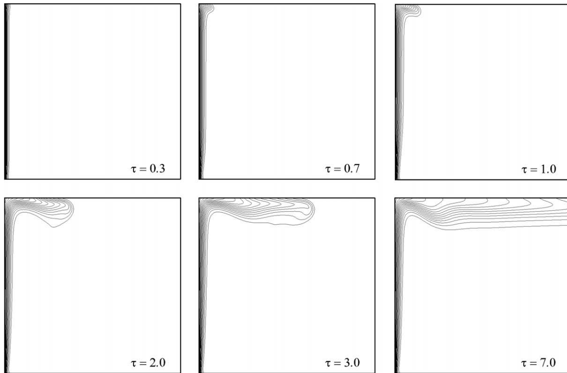
Fig. 2. Numerically simulated temperature contours at the start-up stage (top row) and the steady state (bottom row) of the boundary-layer development at \gamma Ra = 10^7 , Pr = 10 and m = 2 (Case 2), where \tau is the time normalised by H/v_0 .
